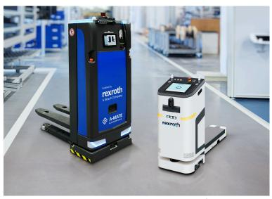
Autonomous, mobile robots such as the ACTIVE Shuttle from Bosch Rexroth and the A-MATE® FreeLift from K.Hartwall can take on joint transport tasks in intralogistics under the VDA 5050-capable ACTIVE Fleet Manager. (Image source: Bosch Rexroth AG)
