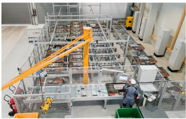
Bosch Rexroth is supplying BLC - The Battery Lifecycle Company with one of the first automation solution for discharging and dismantling battery modules in Europe. (Image source: Bosch Rexroth AG)
