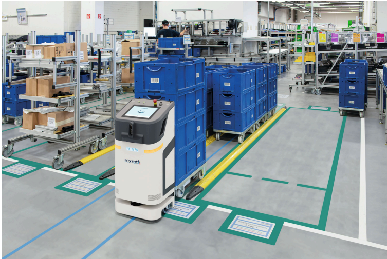
The ACTIVE Shuttle autonomous mobile robot transports small load carriers autonomously, safely and with great flexibility. (Image source: Bosch Rexroth AG)
