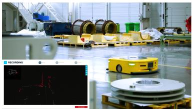
The modular ROKIT toolkit includes software and hardware components for autonomous driving, irrespective of the vehicle architecture or size. (Image source: Bosch Rexroth AG)
