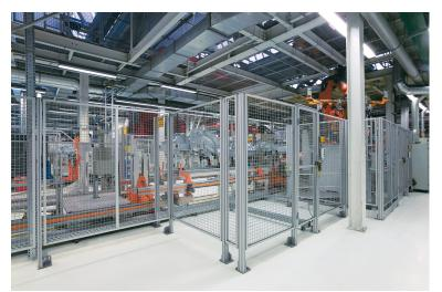
With the EcoSafe material for guards designs from Bosch Rexroth, safety fences can be put in place more quickly and flexibly and at lower cost (Image source: Bosch Rexroth AG)
