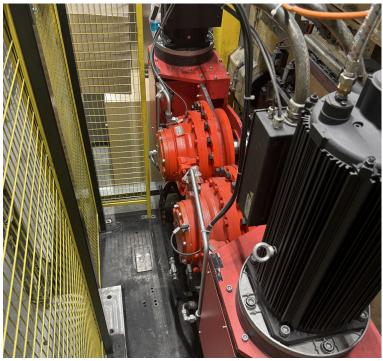
The two roller drives at Freudenberg Sealing Technologies each power 55 kW and use a Hägglunds CA100 hydraulic motor with a rated torque of 25,000 Nm and a nominal speed of up to 23 min-1. (Image source: Freudenberg Sealing Technologies)
