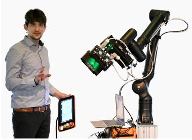
Genuine teamwork: Equipped with Rexroth aluminum profiles, a lightweight robot from Kassow Robots and connecting parts from the PTS Group, the TENTA VISION inspection system can be used in a wide range of applications. (Image source: TENTA VISION)
