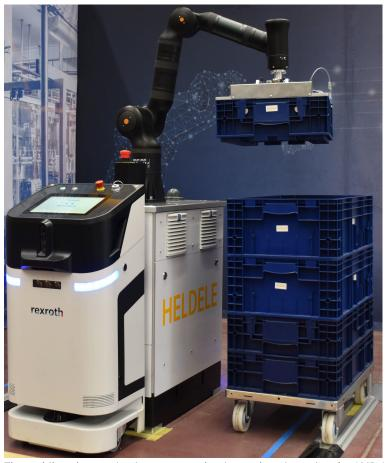
The mobile cobot station is transported to its workstation using the AMR ACTIVE Shuttle from Bosch Rexroth and receives information from the production control system. The KR810 7-axis lightweight robot then begins its work autonomously. (Image source: HELDELE Automation GmbH)
