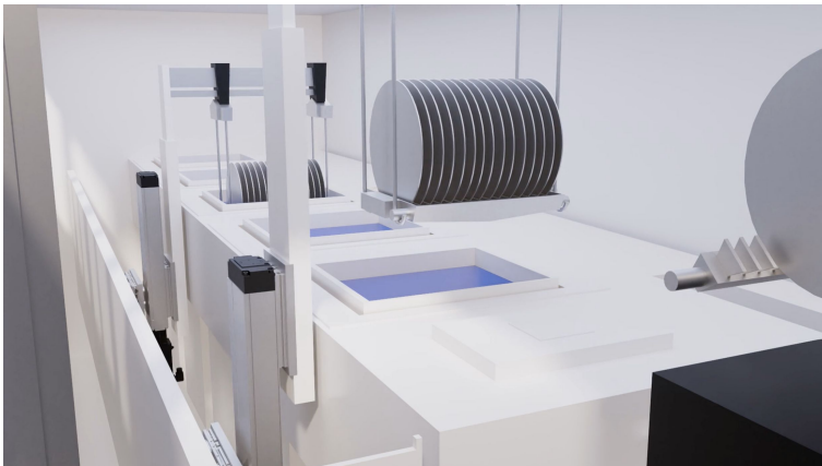
Wafer batch cleaning with mechatronic multi-axis system including motor, drive, and control (image source: Bosch Rexroth AG)
