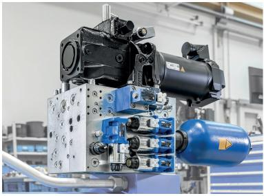
Efficient sheet metal forming: The servo-hydraulic drive solution from Bosch Rexroth increases the energy efficiency of deep drawing presses. (Image source: Bosch Rexroth AG)
