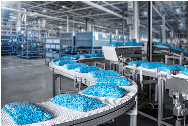
VarioFlow belt conveyor with a very fine-meshed, almost closed and flat surface for FMCG and pharmaceutical/healthcare applications. (Image source: Bosch Rexroth AG)
