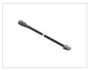
The Ethernet cable consists on the one end of a RJ45 connector and on the other end of a M12 connector, male, 4-pin angular connector, D-coded according to EN61076-2-101. Length approx. 1 m.
