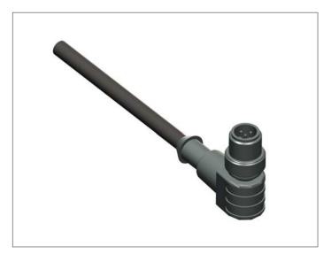
Cable camera mating connector for connection to the wiring harness. The video cable consists of a M12 connector, male, 5-pin, B-coded according to EN61076-2-101 and shows on the opposite side of the cable tin-plated tails. The cable is shielded. Length: approx. 5 m
