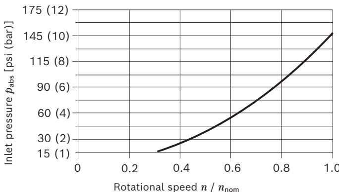
This diagram is only valid for the optimum viscosity range of  $\nu_{\text{opt}} = 36$  to 16 cSt.
