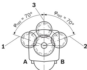
1 "Counter-clockwise" rotation. Pressure at port **B**
