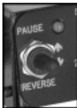
F. To shut off the conveyor when the box is empty, toggle the Pause/Reverse switch back to its centre position.
