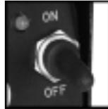
A. Toggle on box power if necessary. Ensure the vehicle is stationary.
