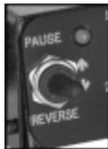
Switched in the upward direction, this function will pause the Spinner and Auger/Conveyor, until switched back to the center position.
