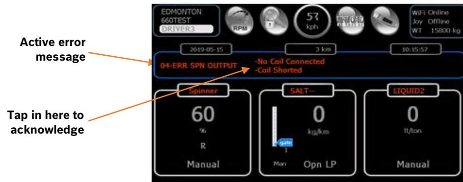
Whenever there are warnings or errors, they are added to a list (log) in the notification area. To clear the log, press and hold anywhere in the rectangle for 5 seconds **with a PGM key inserted**.
