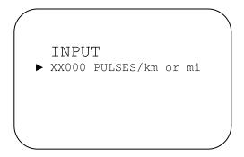
Using the left or right navigation button, move the cursor under the number to be changed.
