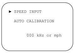
With the cursor arrow pointing at "Speed input" Press Enter and the following screen will appear:
