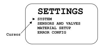
Using the navigation button move the cursor to the area to be configured and press the Enter button.
