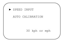
If the speed calibration is off, Press the Enter button to enter the SPEED INPUT phase.
