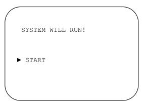
Note: the screen message is a warning that the system will run during the calibration process, make sure all personnel is clear of moving parts. Operate the truck engine at 1500 RPM to ensure good hydraulic oil flow.
