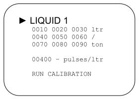
Use the down navigation button to move the cursor to "RUN CALIBRATION" and press the enter button. The following screen will appear:
