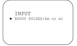
Using the left or right navigation button, move the cursor under the number to be changed.
