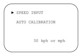
The speed at which you are driving will now be reflected on the screen in the lower, right hand corner.
