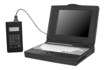
Use this function to transfer all data gathered by the CS-CAL/DLIU from the CS-230 units into a Computer.
