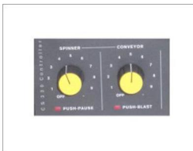
Parameter numbers are selectable by using the spinner and conveyor dials. (For example, setting the spinner dial to 3 and setting the conveyor dial to 5 will show parameter 35 on the screen.)
