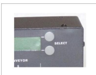
To edit the selected parameter value, press either the upper or lower selector button. The new parameter value will now be displayed on the screen.
