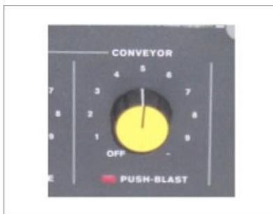
To edit the value of a parameter press the Conveyor dial to go into edit mode.
