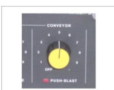
Press the Conveyor Dial again to accept the new parameter and exit edit mode.
