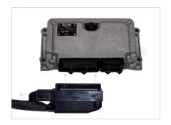
2. Then push in the locking tab and the connector will automatically secure itself.
