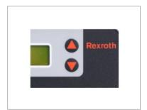
To edit the selected parameter value, press either the upper or lower selector button. The new parameter value will now be displayed on the screen.
