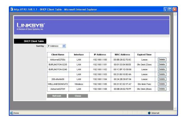
With the IP address the device can be accessed by using the Internet Explore. Similar to the ACC (Airborne Control Centre) the default user name and password is 'dpac'. SSID, Security and static IP address can also be configured on the same screen.
