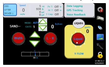
Use the up and down arrows to adjust gate position.
