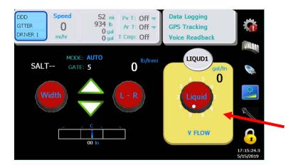
Press & hold on empty spot of the WET panel for 15 secs to Toggle modes
