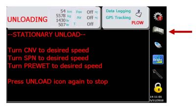
Turn the dials until the desired speed is achieved. Press the symbol again and to exit unload mode. Moving the vehicle will suspend the unload process. It will automatically resume when the truck is stopped again.
