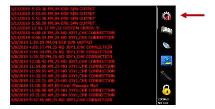
A program key is required to clear the error log; hold the button for >5 seconds.
