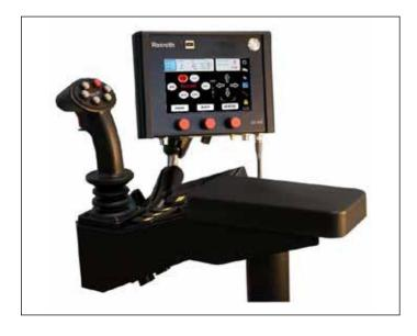
The Rexroth CS-550 controller is designed for multiple Snow & Ice spreader application modes. All controller functions can be viewed on the 7" automotive grade display with glass touch screen. Application rates are controlled by 3 heavily detented knobs; set-up and parameterization is done with the touch screen or a computer.
