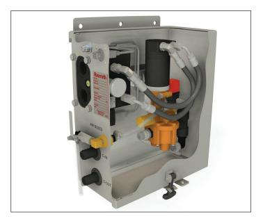
Single ratio pre-wetting module uses return oil from the auger/conveyor motor to drive the pre-wet pump to vary liquid application rates on granular material. A control manifold limits the maximum application rate.
