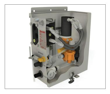
Variable rate pre-wetting module can use return oil from the auger/ conveyor motor to supply the manifold, which controls liquid application rates to the granular material.
