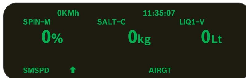
Press the **AIRGT** button to enter the air gate adjustment screen. Press the  $\leftrightarrow$  button to switch between low gate and high gate. The chosen gate setting is highlighted.
