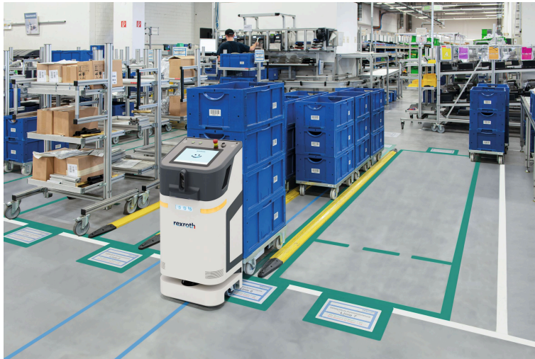
Touchscreen display and 3D obstacle detection: The new ActiveShuttle with Advanced Interaction transports small load carriers autonomously, safely and with great flexibility. (Image source: Bosch Rexroth)
