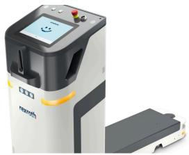
Touchscreen display and 3D obstacle detection: The new ActiveShuttle with Advanced Interaction transports small load carriers autonomously, safely and with great flexibility. (Image source: Bosch Rexroth AG)
