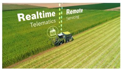
Universal solution for firmware updates over the air: The BODAS Connect Universal Flasher from Bosch Rexroth can update a wide range of control units in off-highway vehicles. This saves time as well as developing, operating and servicing costs. (Image source: Bosch Rexroth AG)
