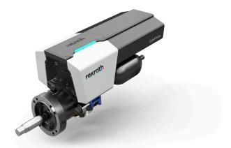
Together with the tank, safety valves and sensors, the CytroForce modules form a highly compact and efficient servo-hydraulic axis with a closed fluid circuit and an energy-on-demand and standardized drive and control concept. (Image source: Bosch Rexroth AG)
