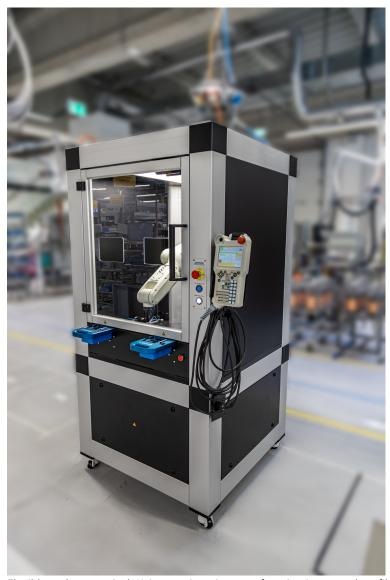
Flexible and economical: Kaiser engineering uses function-integrated profiles from Bosch Rexroth to produce machine enclosures for robotic cells (Image source: Kaiser engineering GmbH)
