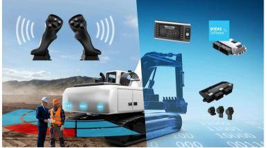
The haptic collision warning system nominated for the bauma innovation award combines hardware and software modules from the BODAS ecosystem for safer, more economical construction machinery. (Image source: Bosch Rexroth AG)
