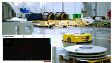
The modular ROKIT toolkit includes software and hardware components for autonomous driving, irrespective of the vehicle architecture or size. (Image source: Bosch Rexroth AG)
