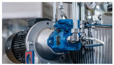
The Sytronix variable-speed pump drives make recycling applications much quieter, more reliable and more energy-efficient. (Image source: Bosch Rexroth AG)
