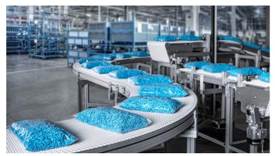
VarioFlow belt conveyor with a very fine-meshed, almost closed and flat surface for FMCG and pharmaceutical/healthcare applications. (Image source: Bosch Rexroth AG)
