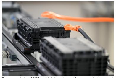
The compact ctrlX CORE, which is based on modern app technology, controls the transfer and the deep discharging process. (Image source: Bosch)
