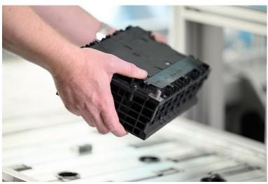
By recycling the batteries, up to 95 percent of the chemical elements can be fed back into the battery production process. (Image source: Bosch)
