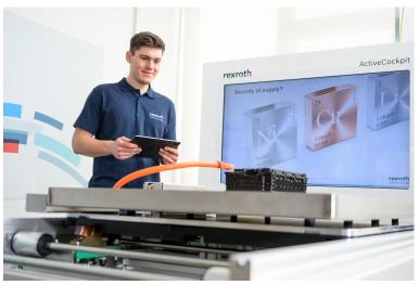
As part of a patented process, an automation solution from Bosch Rexroth takes over the innovative deep discharging of high-performance battery cells. (Image source: Bosch)
