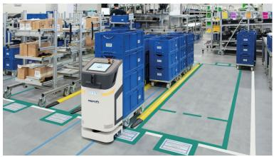
The ACTIVE Shuttle autonomous mobile robot transports small load carriers autonomously, safely and with great flexibility. (Image source: Bosch Rexroth AG)
