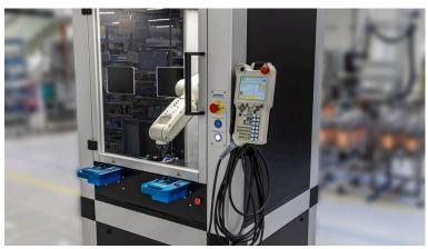
Flexible and economical: Kaiser engineering uses function-integrated profiles from Bosch Rexroth to produce machine enclosures for robotic cells (Image source: Kaiser engineering GmbH)
