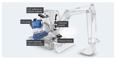
Higher efficiency, better dynamics, individual behavior: With eOC (electronic Open Circuit), machine control, operating feel and dynamics can be set together with other parameters and changed depending on the situation. (Image source: Bosch Rexroth AG)
