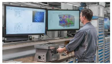
Manifolds from Bosch Rexroth produced using additive manufacturing save resources, energy and CO2. Complementary condition monitoring helps to optimize maintenance costs. (Image source: Bosch Rexroth AG)
