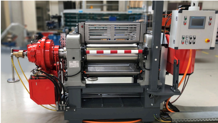
Pre-assembled and tested Hägglunds drive unit for rubber mixing mills of all standard sizes. (Image source: Bosch Rexroth AG)
