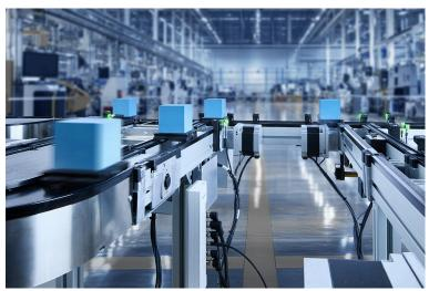
The TS 1 transfer system with compact 48 volt stepper motors allows for small system layouts. (Image source: Bosch Rexroth AG)
