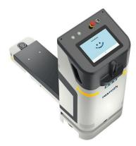
Touchscreen and 3D obstacle detection: the new ActiveShuttle with Advanced Interaction transports small load carriers autonomously, safely and with a high degree of flexibility. (Image source: Bosch Rexroth AG)
