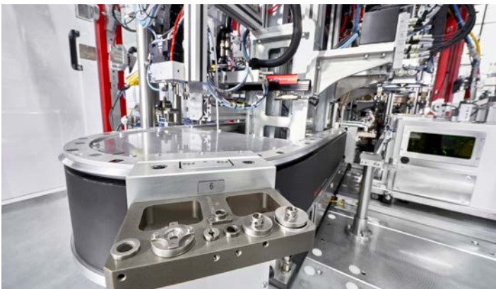
Bosch Rexroth's ActiveMover is a highly dynamic, flexible transfer system based on linear motors. ActiveMover unlocks the potential to increase productivity for small batch sizes, thanks to its quick and precise positioning of workpiece pallets.
