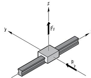
$$(6) F_{\text{comb}} = |F_y| + |F_z| + C \cdot \frac{|M_x|}{M_t} + C \cdot \frac{|M_y|}{M_L} + C \cdot \frac{|M_z|}{M_L}$$
