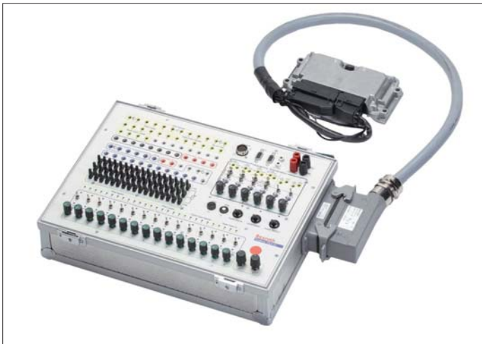
▼ Controller RC36-20/30 connected via TAK4 with two BODAS test boxes TB3/10.
