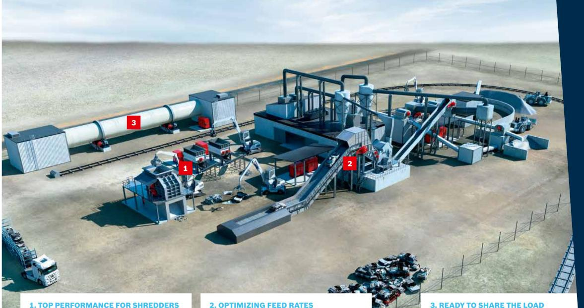
With Hägglunds drives your shredders are a cut above the rest when it comes to reliability. With no gears and no risk of overheating, they can sustain brutal torque - and endure an unlimited number of stops, starts and reversals. When shock loads occur, their hydraulic system instantly relieves stress on shredder bearings and shafts. So teeth and knives stay in service longer, and you can get more done.
