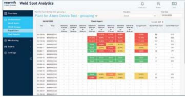
The Rexroth Weld Spot Analytics software package automatically compiles weld spot data into easy-to-read formats and dashboards, enabling an expanded level of real-time analysis and process improvement for welding operations.
