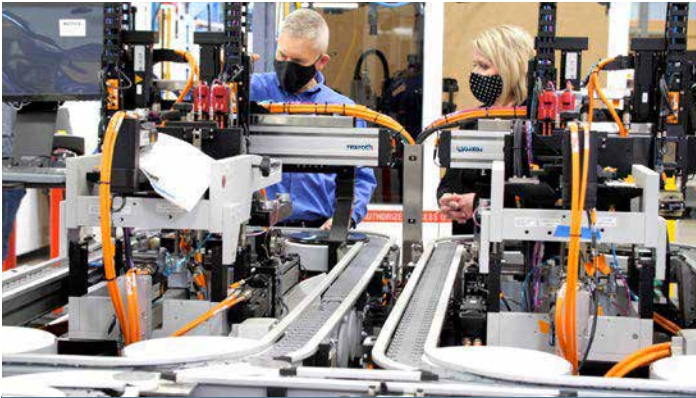
The Rexroth VarioFlow plus flexible chain conveyor system, configured with workpiece pallets, was ideal for the size of the product being manufactured, its weight and the throughput speeds and stopping accuracy required.
