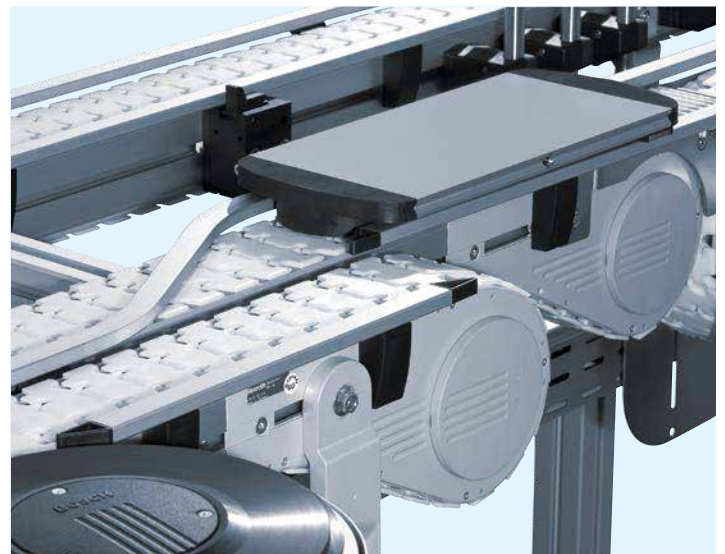
Standardized modular components such as diverters, accumulators, stop units and curve units make it easy to adjust and reconfigure transport layouts based on constantly changing consumer preferences and packaging formats.
